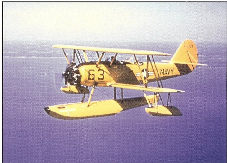
Right: An airborne view of the N3N shows its float and pontoon configuration.
