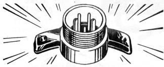
(8) TERMINAL HOUSING ASSEMBLY.—Replace the assembly if the insulator is cracked, if the terminal pins are burned, or if they are bent beyond safe straightening. Replace the heavy leads if the insulation is burned or cracked and peeling.
