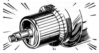
(d) Smooth and polish the commutator to remove any burrs which might have developed from undercutting the mica. Use a fine grade sandpaper, No. 000.
