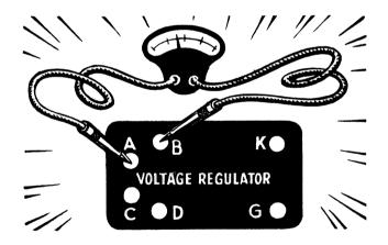
(3) At the end of 30 minutes the value of the "control resistor volts" must not be less than shown in the following table:
