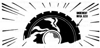
(c) After turning, carefully undercut the mica to a depth of .020 of an inch. Use a cutting tool slightly wider than the thickness of the mica (.020 of an inch), to insure complete removal of the mica to the required depth.
