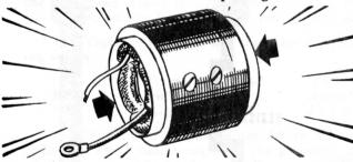
(9) FIELD COIL INSULATORS.—If the insulating strips at each end of the field ring assembly are damaged, they should be replaced.
